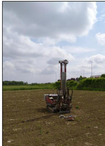
**Figura 8.2.2** – Foto prove penetrometriche CPT3-CPT4
